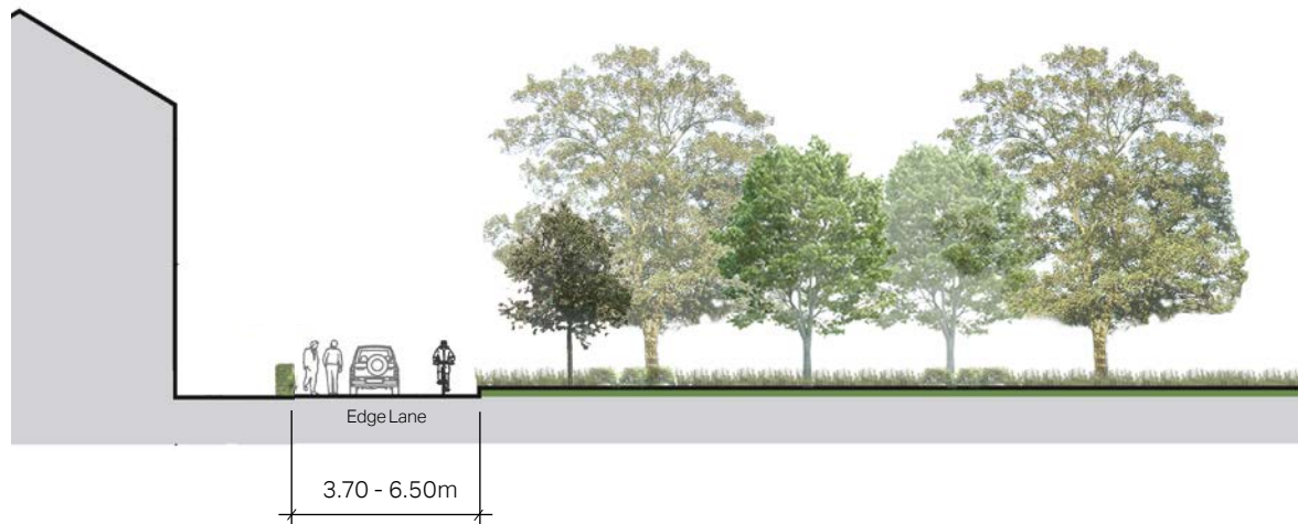
Figure 86: Cross-section to illustrate some dimensions for edge lanes.
