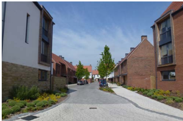
Figure 81: Tertiary street with inset parking bays alternating with trees on both sides, elsewhere in UK.
